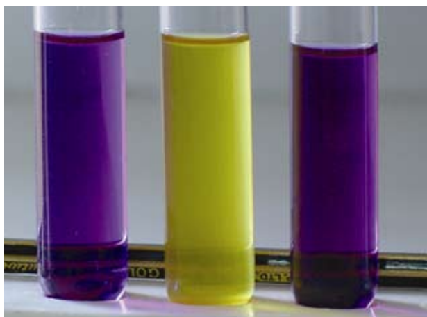
Figure 4: Glucose Azide Broth with bromo cresol purple as indicator (left control, middle positive reaction, right negative reaction)
